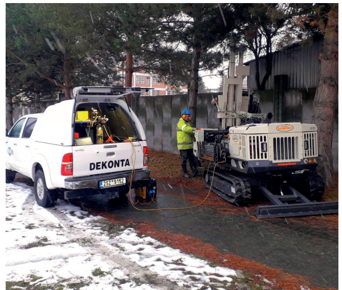
MIHPT logging using Geoprobe 7822DT
